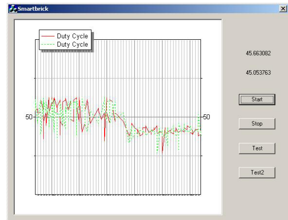
Figure 3: Sample screenshot of real-time data collection software, with traces of X and Y-axis acceleration measurements. The horizontal axis is time and the vertical the duty cycle of the acceleration signals. A duty cycle of 50 indicates a neutral 0.0g alignment.
