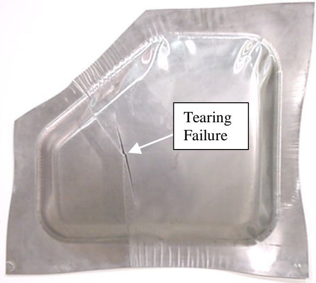
FIGURE 5. FULL VIEW OF NON-SYMMETRIC TEST PANEL WITH SEVERE TEARING FAILURE AT A DEPTH OF 80-MM USING A TRADITIONAL FORMING PROCESS.
