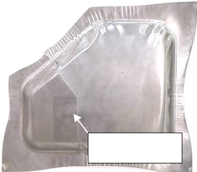
FIGURE 8. MINOR ENGINEERING STRAINS IN THE THINNER MATERIAL ALONG THE SLANTED WELD LINE AND VERTICAL WELD LINE..
